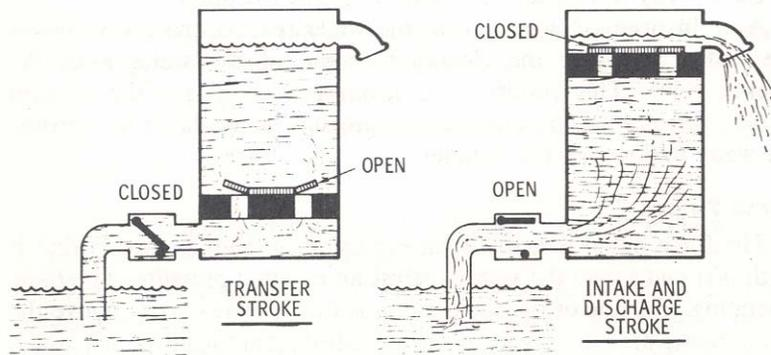
The force pump is another type of reciprocating pump. It actually lifts and forces the water against an external pressure. In a force pump, water is drawn into a cylinder in the
