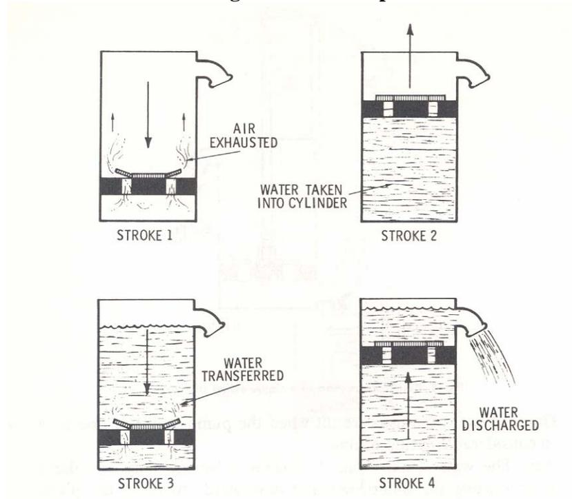
**Fig. 4. Four-stroke starting cycle for a single-acting lift pump.**
