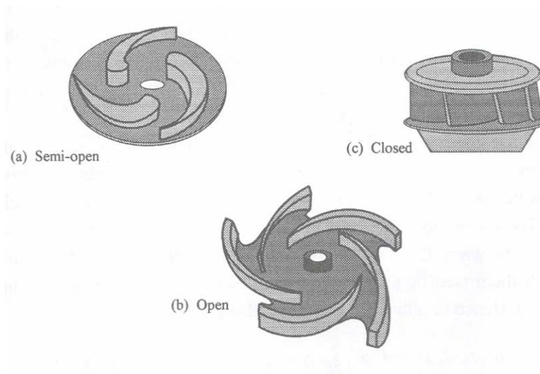
The closed impeller uses a front and back shroud to leave only the suction eye and outer edge of the impeller open. The closed impeller is generally used for pumping clean water or water with minimum solids such as treated wastewater and can generate very high pressures.
