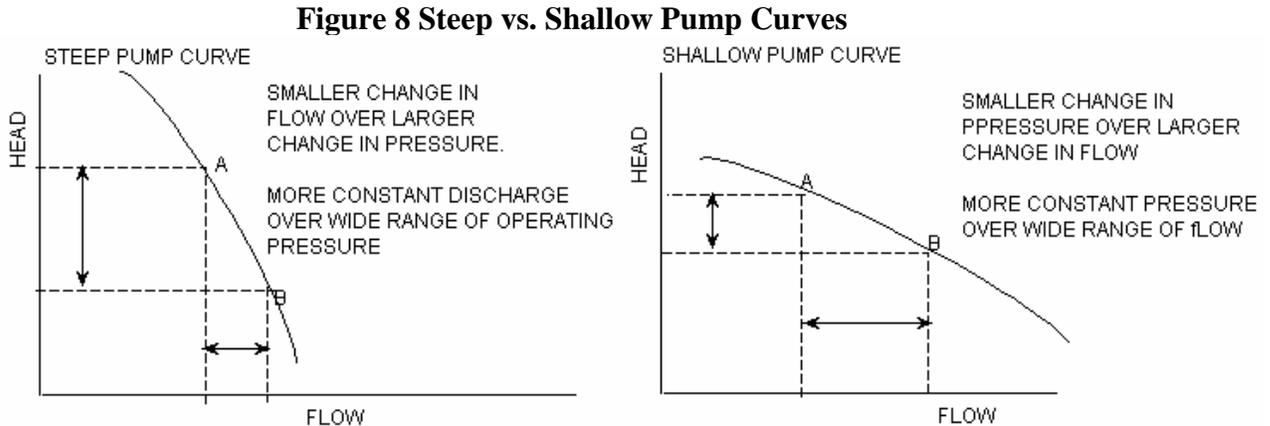
Unpredictable variations in flows can pose difficult problems for low-pressure sewers because the increase in flows will cause an increase in head losses through the system. To overcome this potential problem, low-pressure sewers often use pumps with steep head curves as shown below in Figure 8. The pump described in Figure 8 will deliver between 8 and 14 gallons per minute with pressures ranging from 0 to 60 psi. A steep pump curve will provide a stable flow over various pressures.
